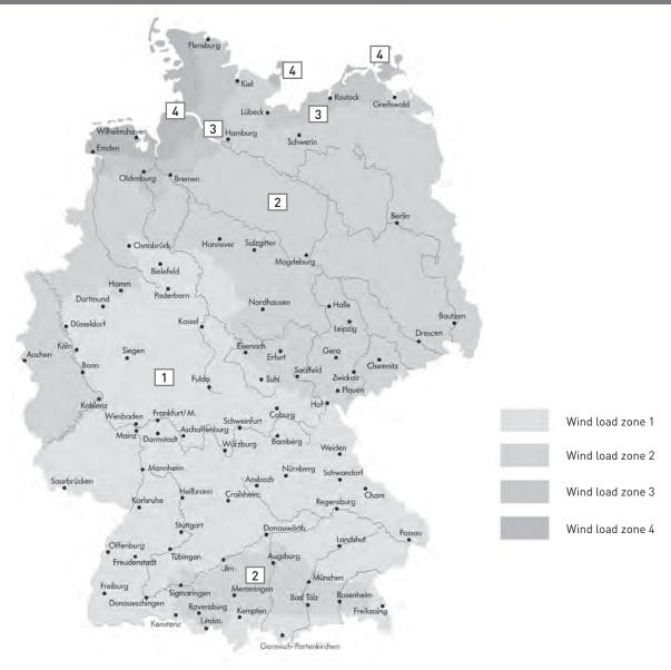
Read off the wind load zone from the map. In borderline cases, always choose the higher zone! Determine the terrain category using Table 1. Read off the wind resistance class from Table 2.
